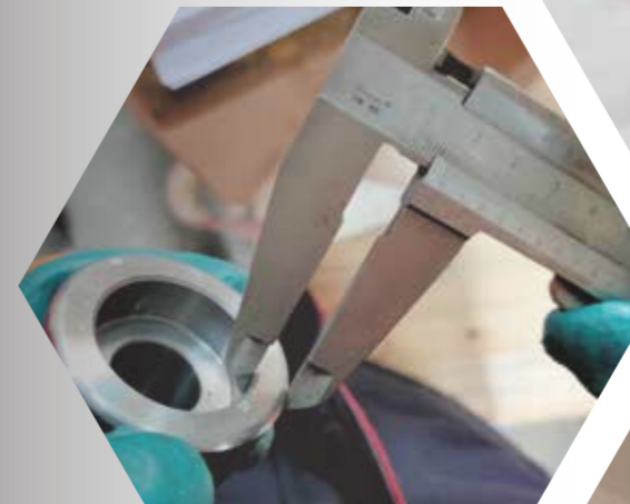
Measuring Wall Thickness
